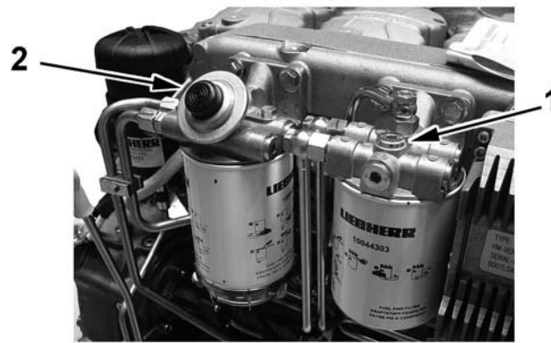
Bleed screw on the filter head of the fuel fine filter
