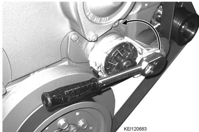
Mounting the ribbed V-belt with tensioning device
